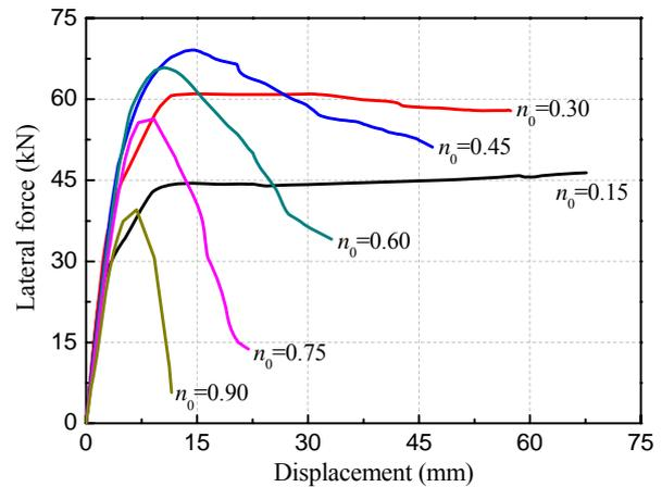
Fig.3 Predicted lateral responses with different preloading stress level indexes
