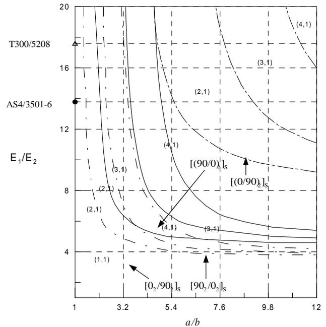
Fig.1 Boundary of thermal buckling mode for simply supported cross-ply laminates.
