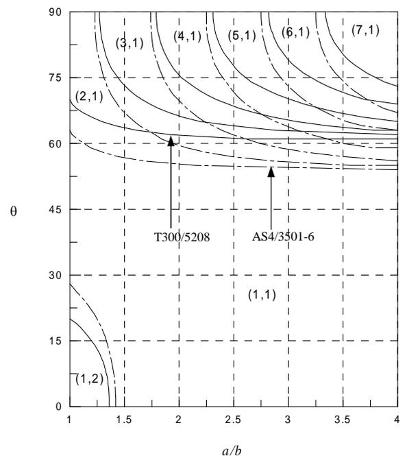
Fig. 2 Boundary of thermal buckling mode for simply supported  $[(\pm\theta)_2]_s$  angle-ply laminates.
