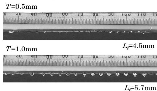
Figure 2 Effect of EVOH sheet thickness,  $T$ , on the formation of the Taylor cone.
