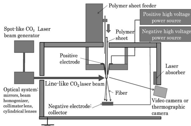
Figure 1 Schematic diagram of the line laser melt electrospinning system used in this work.
