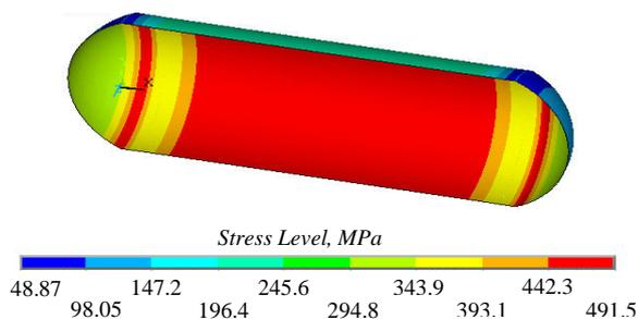
Figure 1 reveals that the stresses develop in the aluminum liner reach a magnitude of 491.5 MPa at the interior surface of the tank, which exceed the tensile strength of the aluminum liner, 310 MPa (Boresi and Schmidt, 2003). This qualitatively agrees with experimental results published by Dubno (2006) who built and tested a tank prototype that failed at internal pressure of 410 bars versus an expected burst pressure of 804 bars.
