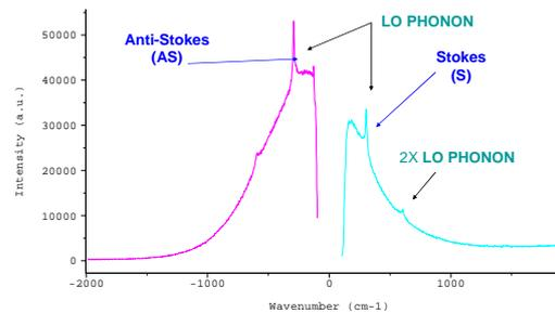
Figure 1. Raman spectra of CdS nano-rods of 1.7 nm and of diameter and 10 nm length, exhibiting unusual intensity ratio of anti-Stokes to Stokes, at low temperature. Also shown are the relevant second order phonon scattering. The background is the relevant photoluminescence emission. The exciting laser wavelength is 488 nm of the argon lase
