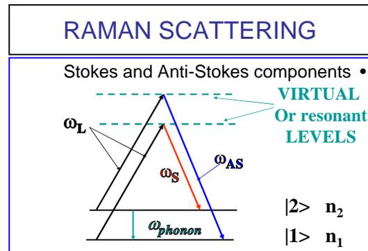
Figure 2. Raman scattering scheme showing the Stokes and anti-Stokes components and the phonon levels.
