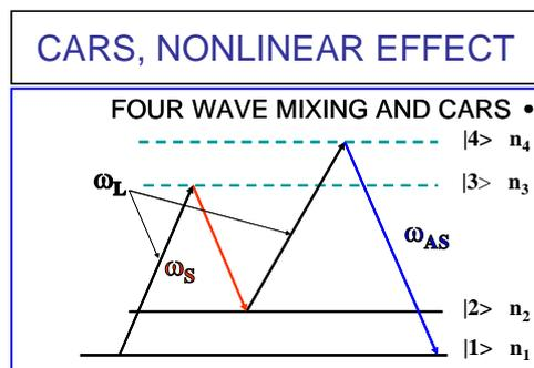
Fig. 3 CARS nonlinear model. In the present experiment two laser photons and one Stokes photon generates the fourth anti-Stokes photon in a four wave mixing process.
