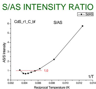
Figure 4. Results of measured Stokes to anti-Stokes intensity ratio in the temperature range of 100 °K to room temperature. Notice the unusual "inverted" ratio in most of the temperature range of the experiments.
