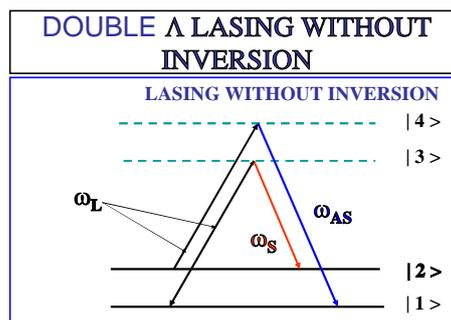
Figure 5. The coherent two laser photons and the Stokes photon generates a lasing without inversion in a double Lambda scheme, via a quantum interference process.
