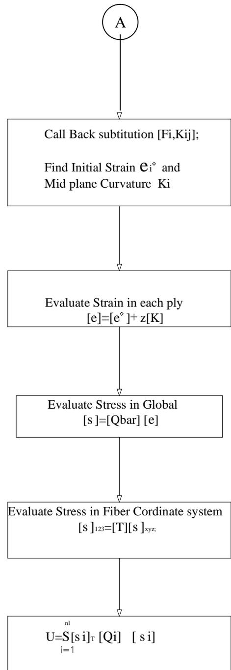
Basic Flow Chart To Find Stresses, Strains and Strain Energy
