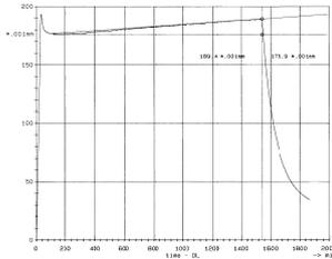
Fig. 4 Course of relative elongation of the piston sample, as a function of time for the aging at a temperature of 200°C.
