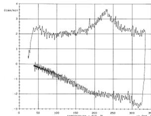
Fig 5 The course of derivative of specimen dimension increase to the time as a function of temperature (T) during heating and cooling (phase transition in 170°C-300°C temperature range).
