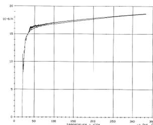
Fig. 7 The linear course of the coefficient of linear expansion  $\alpha$  as a function of temperature (T) during heating and cooling with a minimum difference of coefficient at the same temperature.
