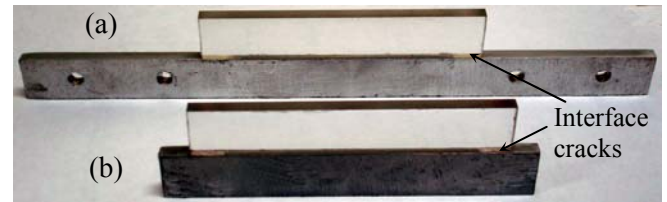
Fig. 1 Bimaterial specimens with interface edge cracks shown for (a) bending (b) convection-cooling.
