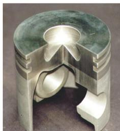
Fig. 3: Composite piston locally reinforced.
