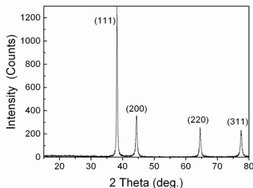
Fig.1 XRD pattern of the prepared particles
