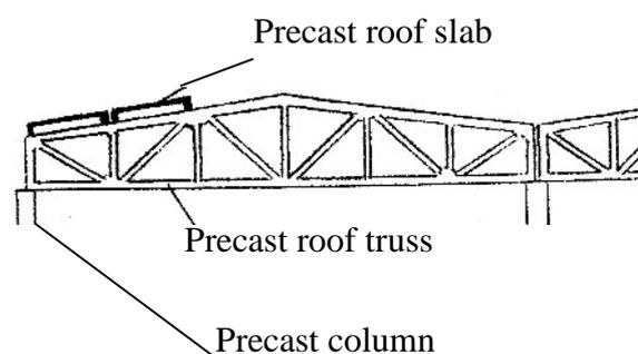
Fig. 1 Steel-concrete composite precast and prestressed roof trusses accommodating roof precast slabs and supported by precast columns
