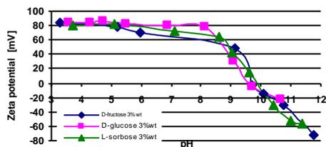
Fig. 1 Zeta potential measurements of nanosized alumina suspension with addition of 3 wt.% of monosaccharides
