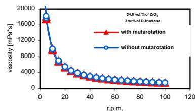
Fig. 3 Influence of 3wt% fructose concentration on viscosity of n-ZrO<sub>2</sub> suspension at shear rate 33 s<sup>-1</sup>, monosaccharide were added before and after mutarotation
