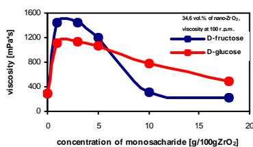
Fig. 2 Influence of monosaccharides concentration on viscosity of n-ZrO<sub>2</sub> suspension at shear rate 33s<sup>-1</sup>
