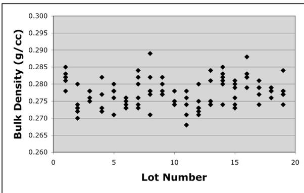
Figure 2: PICA Billet Bulk Density Repeatability
