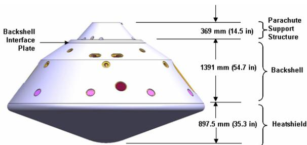
Figure 1: MSL Aeroshell Configuration
