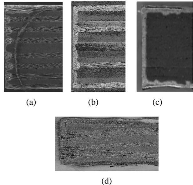
Figure 2: Dark-field images of oxidation in a (a) cross-ply, (b) quasi-isotropic, (c) angle-ply and (d) plain-weave composite
