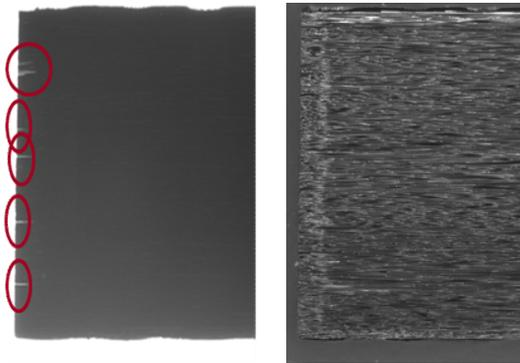
Figure 1: Optical microscopy images in a cross section parallel to the  $0^\circ$  direction in  $[0]_{16T}$  laminate
