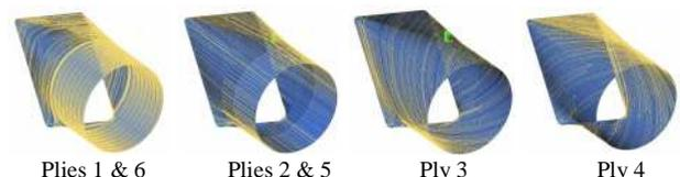
Figure 3: Ply Prepreg Duct Laminate Definition
