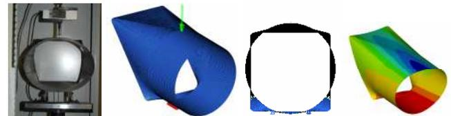
Figure 2: Experimental set-up showing wet lay-up woven fabric duct in fixture (on left), FEA model of loads and supports (center), and deflection contours (on right)
