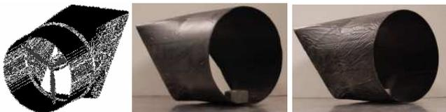
Figure 1: CAD rendering of duct along with prepreg (center) and wet lay-up (right) prototypes
