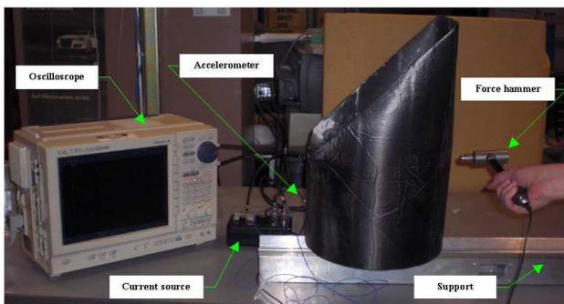
**Figure 4: Experimental set-up for dynamic analysis**
