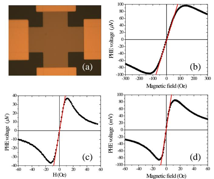
Fig. 1 (a) Micrograph of the single  $50\ \mu\text{m}\times 50\ \mu\text{m}$  PHE sensor junction, (b)-(c) the PHE profiles of the bilayer structure, spin-valve structures and bilayer structure with a thin spacer layer between AF and FM layers.
