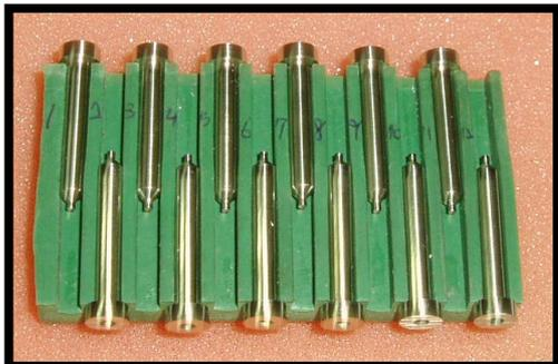
Fig. 3 Micro tubes for the micro hot runner module
