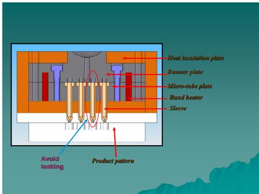
Fig. 1 Schematic drawing of a micro hot runner module
