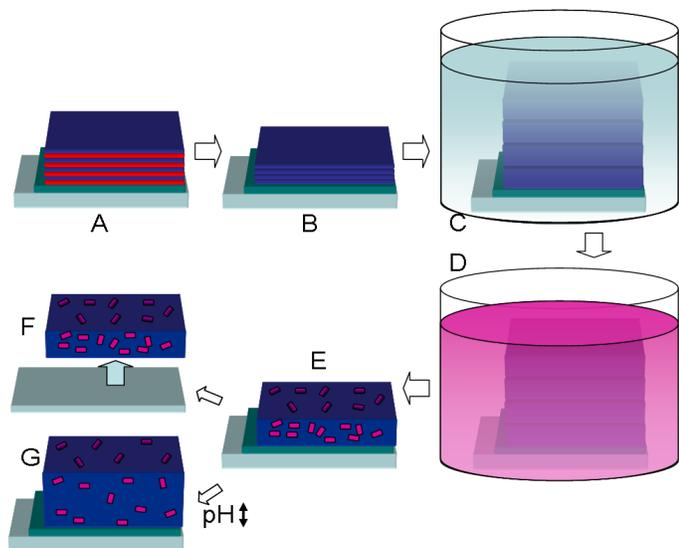
Fig. 3. Schematics of fabrication of layered hydrogels with gold nanorods.
