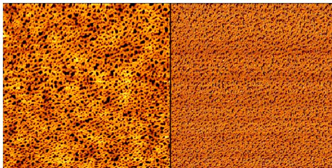
Fig. 2. AFM image (topography and phase) of nanoperforated LbL film.
