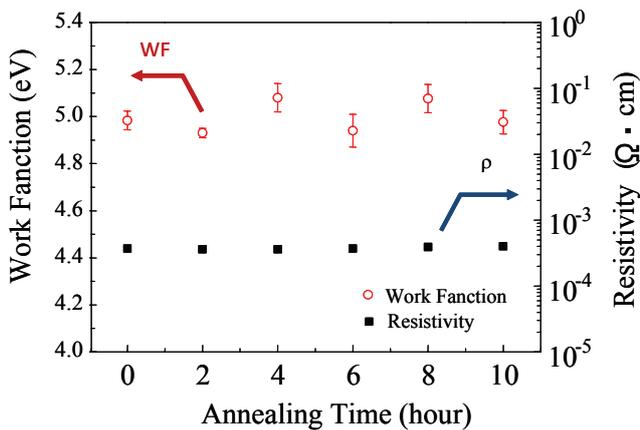
Fig. 2 WF and Resistivity dependency on annealing time for PEN substrate with ITO.
