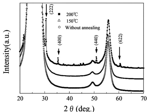
Fig.1 X-ray diffraction patterns of PEN film with ITO.
