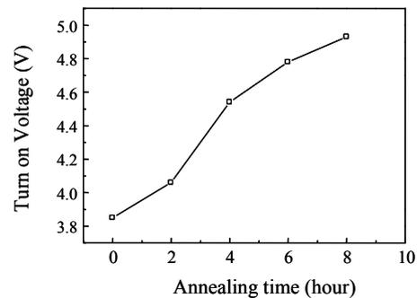
Fig. 4 The turn-on voltage (@1cd/m<sup>2</sup>) vs annealing time for PEN substrate with ITO .
