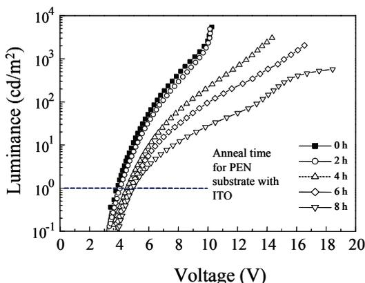
Fig. 3 Luminance-voltage (L-V) characteristics of OLEDs.
