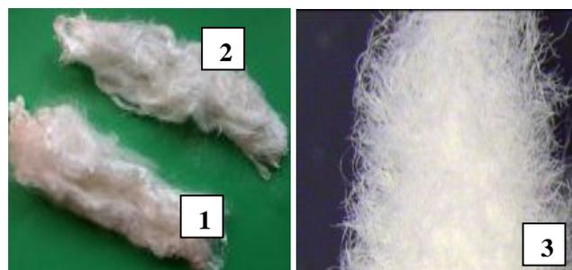
Fig.1 The initial cellulose fibers (1), oxide fibers (2), triple composite fibers Al<sub>2</sub>O<sub>3</sub>-ZrO<sub>2</sub>-Y<sub>2</sub>O<sub>3</sub> (3)
