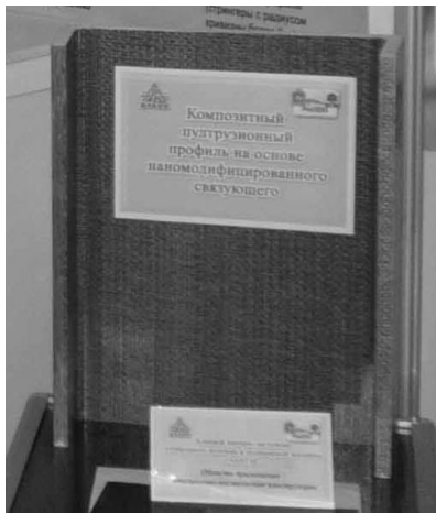
Fig.1: Glass fiber U-profile 400 120 18mm on the base of vinyl ether resin with nanocuprum
