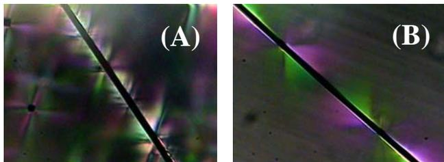
Fig.1 Typical fragmental images of CFs. (A): CO<sub>2</sub>/H<sub>2</sub>O treated CF; (B): Other treated or untreated CFs.
