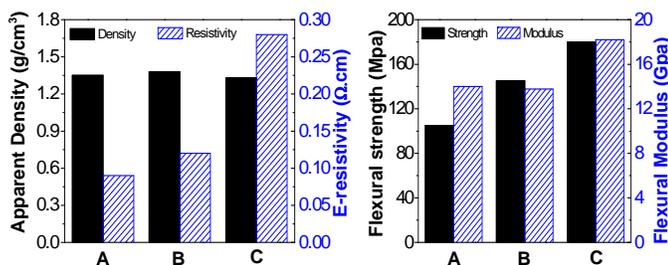
Fig. 2 Physical properties of CFCs. A: UTSI CF; B: HNO<sub>3</sub> treated CF; C: O<sub>3</sub> treated CF.
