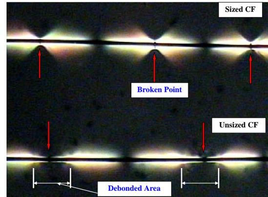
Fig. 3 Fragmentation tests comparing sized CF with unsized CF in epoxy resin.
