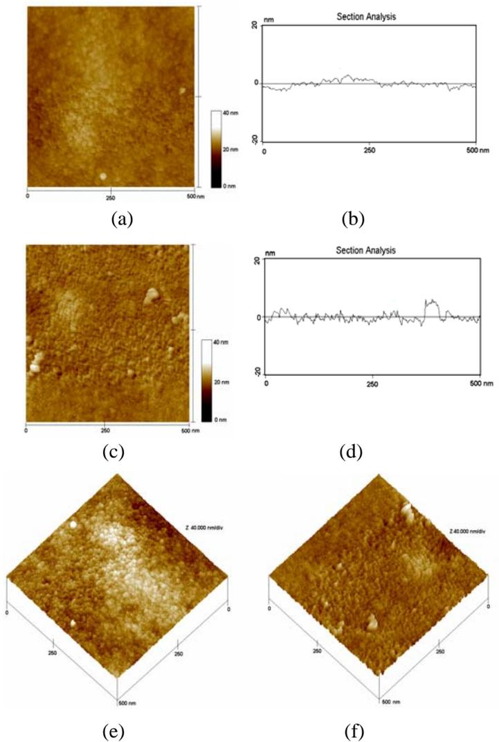
**Fig. 2** Top-view AFM images of Ag/TiO<sub>2</sub> calcined at (a) 100 °C, (b) line profile (c) 400 °C, (d) line profile, (e) 3D (100 °C) and (f) 3D (400 °C).
