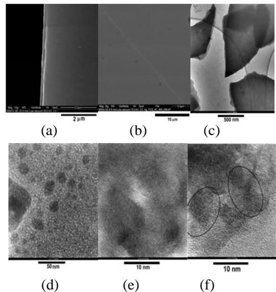
**Fig. 3** (a) and (b) SEM of the films calcined at 100 °C, (c) and (d) TEM of the films calcined at 100 °C, (e) and (f) HRTEM of films calcined at 400 °C.
