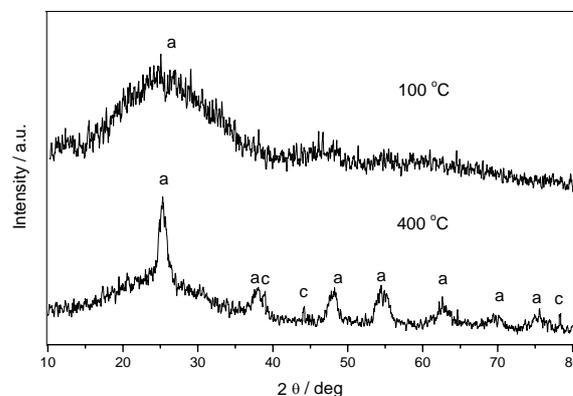
**Fig. 1** X-ray diffraction patterns of Ag/TiO<sub>2</sub> calcined in indicated temperatures (a=anatase and c = metallic Ag).
