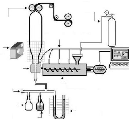
Figure 1. Schematic diagram of the film blowing experimental set-up.
