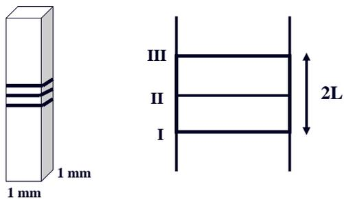
Figure 3 Specimen dimension
