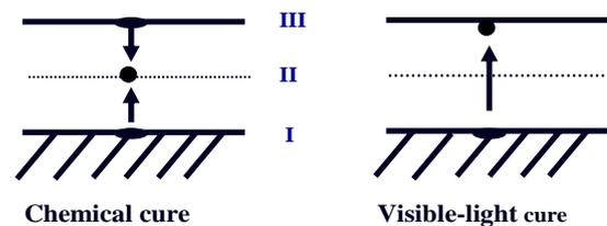
Figure 2 The formation of microcracks
