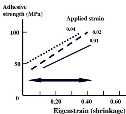
Figure 5 Adhesive strength in chemical cured sample
