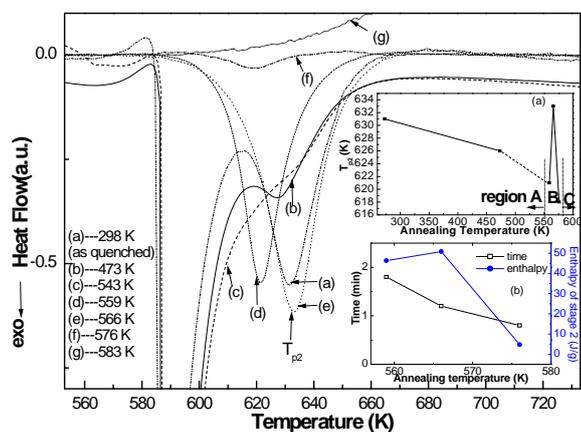
Fig. 2 DSC scans for  $\text{Al}_{83}\text{Ni}_{10}\text{Ce}_7$  metallic glass in stage 2 after isothermal annealing
