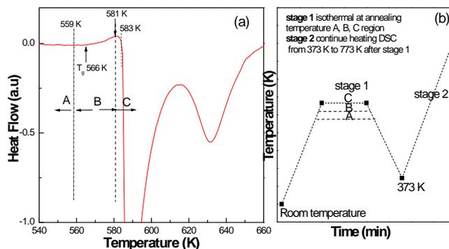
Fig.1 DSC scan (a) of  $\text{Al}_{83}\text{Ni}_{10}\text{Ce}_7$  metallic glass at a rate of 20 K/min
