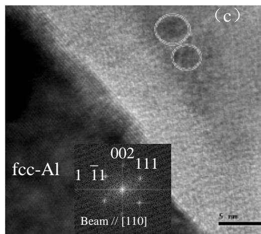
Fig.3 HRTEM image (a) of the as-quenched  $\text{Al}_{83}\text{Ni}_{10}\text{Ce}_7$  glass; TEM bright-field image (b) and HRTEM images (c)
