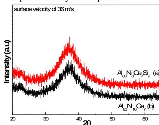
Fig.1. XRD patterns for melt-spun  $\text{Al}_{83}\text{Ni}_8\text{Ce}_7\text{Si}_2$  (a) and  $\text{Al}_{83}\text{Ni}_{10}\text{Ce}_7$  (b) ribbons, showing an amorphous structure at surface velocity of 36 m/s
