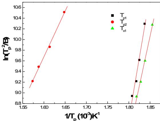
Fig. 3 Kissinger plots between  $1/T_p$  and  $\ln(T_p^2/B)$  of amorphous  $\text{Al}_{83}\text{Ni}_8\text{Ce}_7\text{Si}_2$  alloy.
