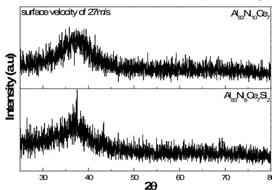
Fig. 2 XRD patterns for melt spun  $\text{Al}_{83}\text{Ni}_8\text{Ce}_7\text{Si}_2$  and  $\text{Al}_{83}\text{Ni}_{10}\text{Ce}_7$  ribbons at a surface velocity of 27 m/s.
