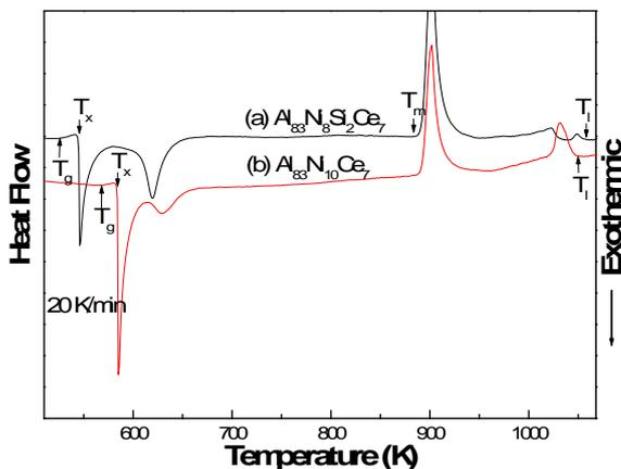
Fig. 4 DSC curves of as-spun  $\text{Al}_{83}\text{Ni}_8\text{Ce}_7\text{Si}_2$  (a) and  $\text{Al}_{83}\text{Ni}_{10}\text{Ce}_7$  (b) ribbons at a heating rate of 20 K/min.
