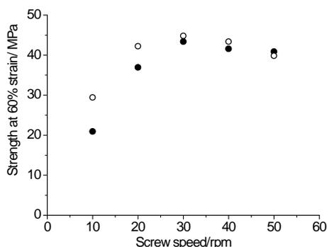
Fig. 3 A plot of tensile strength versus extruder screw speed for polyethylene specimens that have been extruded in the presence (open circles) and absence (solid circles) of ultrasound.
