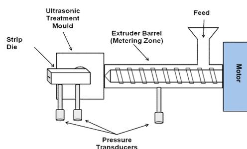
Fig. 1 Schematic of the in-line ultrasonic extrusion set-up.
