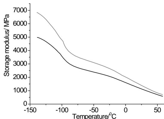
Fig. 4 DMA results for specimens of the PE80 blend that have been extruded in the presence (gray line) and absence (black line) of ultrasound.
