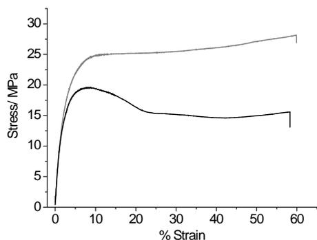
Fig. 2 Stress-strain curves for specimens of the PE80 blend that have been extruded in the presence (gray line) and absence (black line) of ultrasound.
