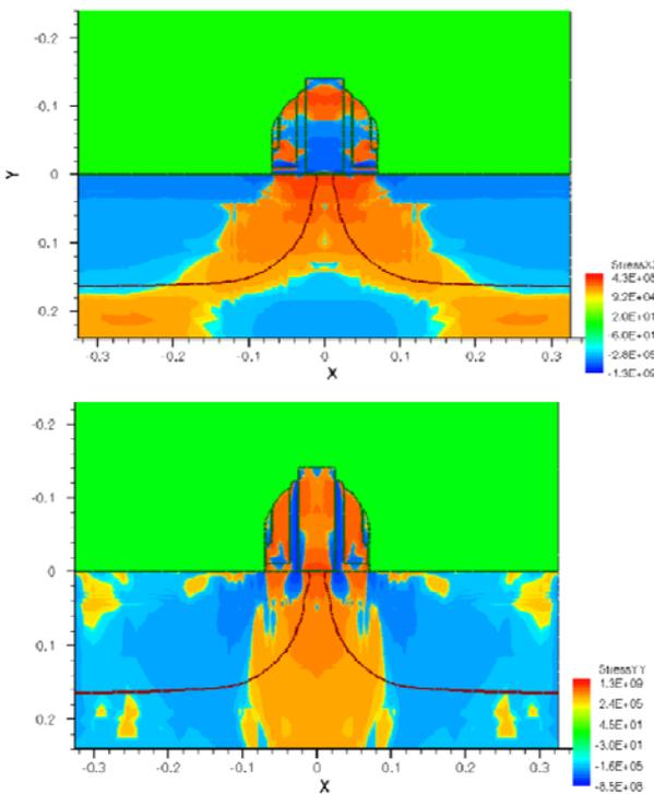
Fig. 3 Contour plot of (a)  $\sigma_{xx}$  (Pa) and (b)  $\sigma_{yy}$  (Pa) after  $\text{SiN}_x$  stressor etch. All lengths are in  $\mu\text{m}$ .
