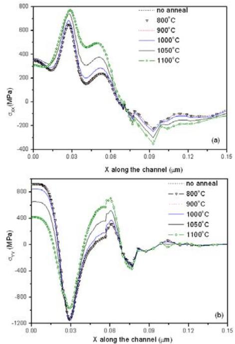
Fig. 4 Channel stress  $\sigma_{xx}$  (a) and  $\sigma_{yy}$  (b) at 1nm below Si surface for different anneal temperatures
