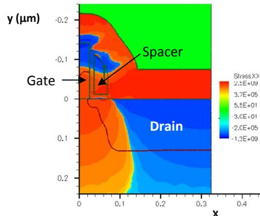
Fig. 1 Contour plot of  $\sigma_{xx}$  (Pa) after  $\text{SiN}_x$  deposition
