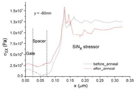
Fig. 2 Stress profile of  $\sigma_{xx}$  before and after rapid thermal anneal at  $1050^{\circ}\text{C}$  for 1s
