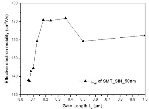
Fig. 5 Extracted effective electron mobility versus polysilicon gate length of SMT nMOSFETs.
