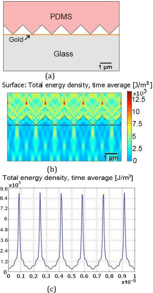
Fig. 2 (a) Schematic of a phase-shifting PDMS mold and a Au thin film coated substrate used in simulation; (b) Diagram of light intensity distribution; (c) Energy density distribution on the gold surface.
