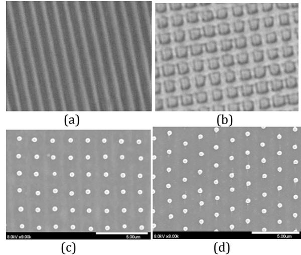
Fig.3 Photothermal annealed periodic nanostructures (line-line and particle-particle spacing is 5/3μm). (a) gold nanowires; (b) 1×1μm<sup>2</sup> gold square before flood exposure; (c) 400 nm diameter gold nanospheres form orthogonal array after flood exposure; (d) Hexagonal gold nanosphere array (bar = 5μm).
