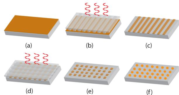
Fig.1 Schematic of NPTA processes. (a) A thin gold film is coated on a glass slide; (b) A 1-D grating PDMS mold is placed on top of a gold thin film followed by laser pulse illumination; (c) Gold nanowires form after exposure; (d) Rotate the PDMS mold and repeat process (b); (e) Isolated gold squares form; (f) Gold squares bead up and form nanospheres after flood laser exposure
