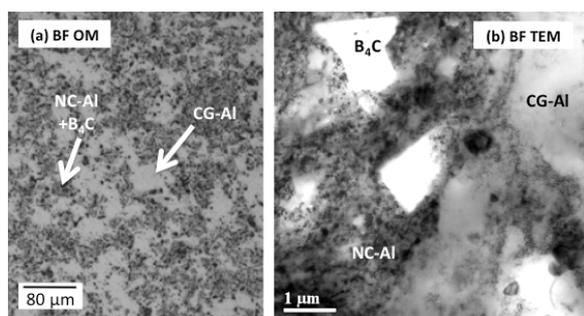
Fig. 2. The multi-scale microstructure of tri-modal Al MMCs examined by (a) optical and (b) TEM bright-field.
