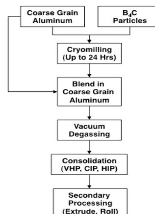
Fig. 1. Manufacturing processing of tri-modal Al MMCs.
