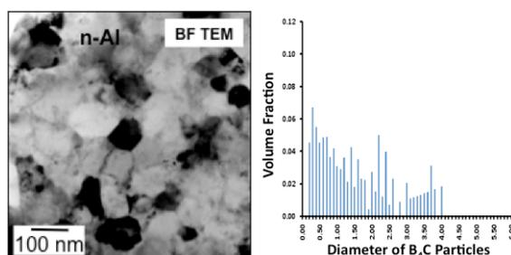
Fig. 3. Typical grain microstructure of NC-Al and particle size distribution of B<sub>4</sub>C in trimodal MMCs.
