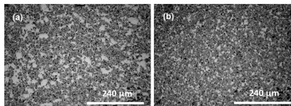
Fig. 4. Trimodal MMCs with variation in CG-Al and cryomilled agglomerate domain size.
