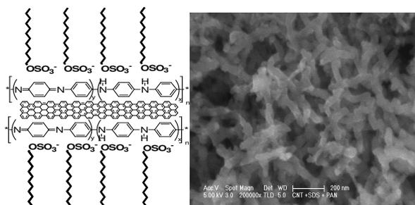
Fig.2: Schematic description [left] and SEM image [right] of the composite SWCNT/SDS/PANI synthesized by *in situ* chemical polymerization.
