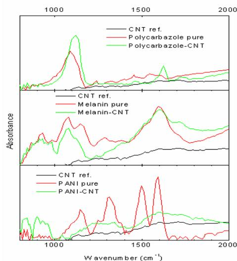
Fig.1: IR spectra of the hybrid materials (conducting polymers coated SWCNT) and their constituents.
