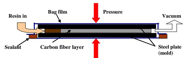
Fig. 2 Vacuum bagging resin infusion for making CFCs
