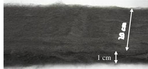
Fig.1 Typical UTSI carbon fiber form
