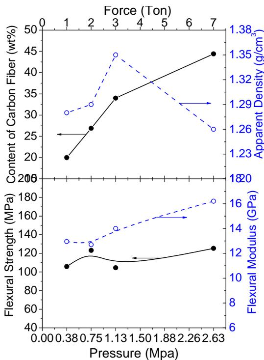
Fig. 3 Effect of applied pressure on physical properties of the epoxy CFCs
