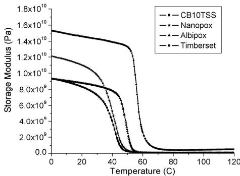
Fig.2: Storage modulus versus temperature for all the adhesives.
