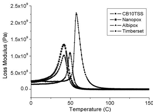
Fig. 3: Loss modulus versus temperature for all the adhesives.
