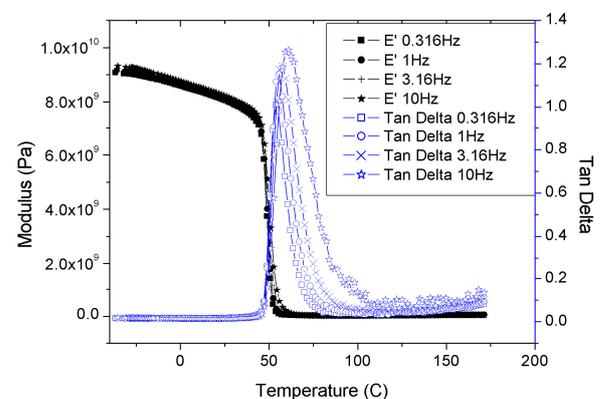
Fig.1: Graph of Modulus and Tan Delta versus temperature at four frequencies for Albipox.
