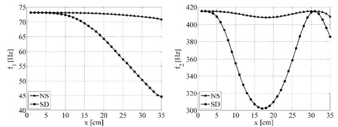
Fig. 6 Influence of simulated damage on values of the first (left) and second (right) eigen-frequencies for cantilever sandwich beam.
