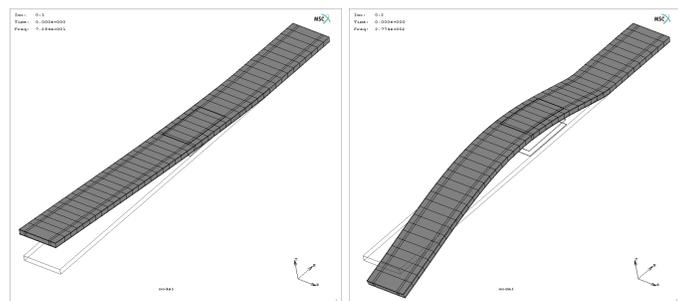
Fig. 5 First two eigen-modes of cantilever hybrid beam.
