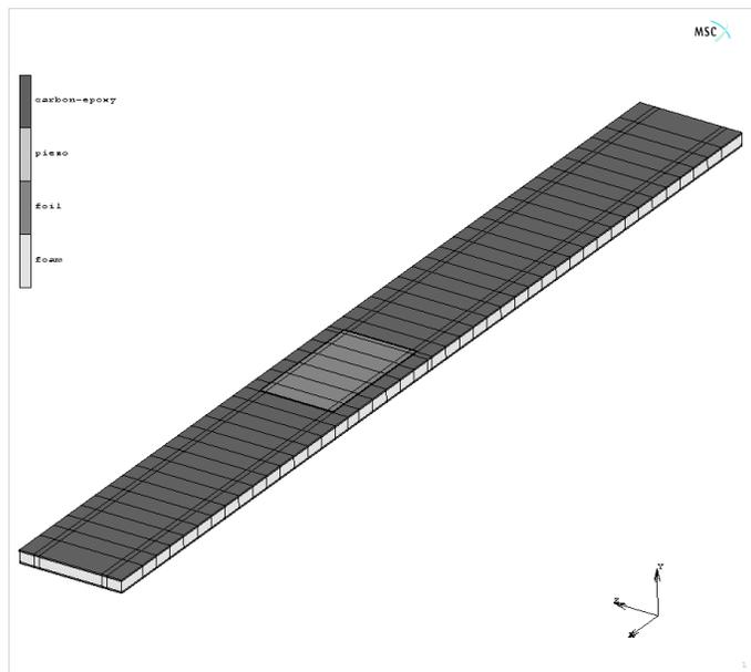
Fig. 4 Finite element model of hybrid sandwich beam.
