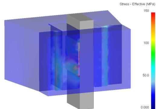
Fig. 4 ASF\_3D\_04: Loading of assembly during the first pass.
