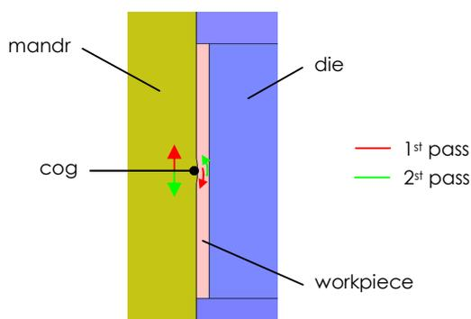
Fig. 1 Principle of ASF process.
