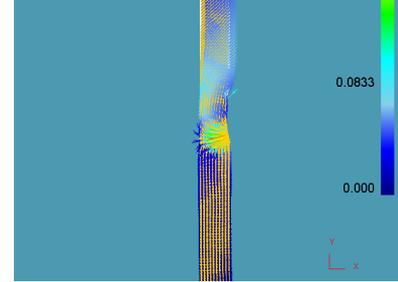
Fig. 3 ASF\_2D\_05: Material flow during the first pass.
