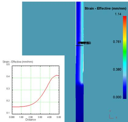
Fig. 2 ASF\_2D\_05: Effective strain in work-piece after the first pass.
