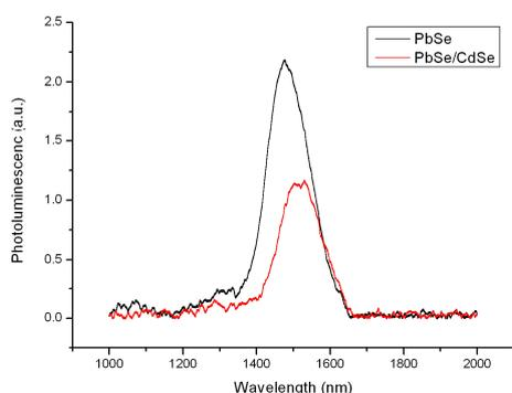
Fig.2: The evolution of the photoluminescence spectra of 4.8 nm PbSe cores with 2.1 nm CdSe shell
