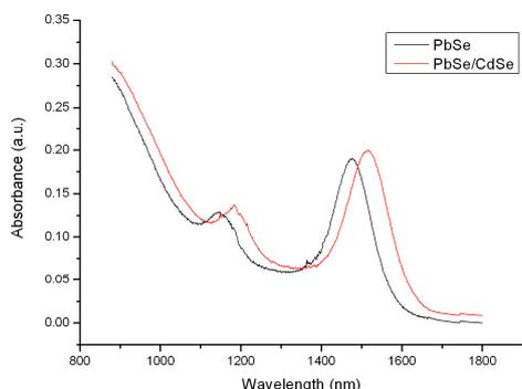
Fig.1: The evolution of the absorption spectra of 4.8 nm PbSe cores with 2.1 nm CdSe shell.
