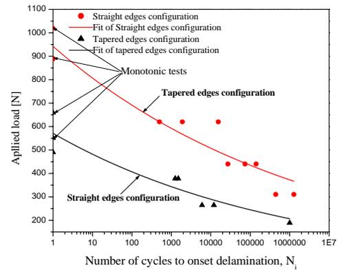
Fig. 3 Maximum cyclic load as a function of the number of cycles to delamination onset for both configurations.
