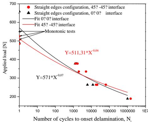
Fig. 2 Maximum cyclic load as a function of the number of cycles to delamination onset for Straight edges.
