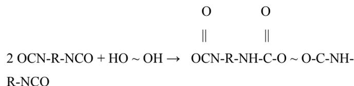
This prepolymer - Component B - further interacts with other agents of polyurethane composition (component A), participating in the reaction of the growth of the polymer chain. Component A contains the remainder of the polyester, chain extender, foaming agent, catalyst, emulsifier, pororegulator and ink pasta.
