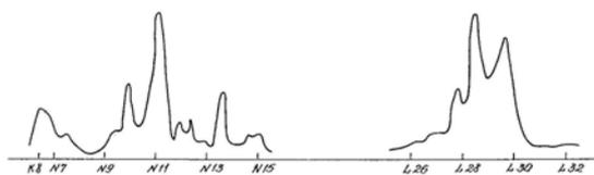
Found that in ether (Part A) spectra of ether were found at frequencies of 1000-1120 cm<sup>-1</sup>, amide group at 1370 cm<sup>-1</sup>, CHs-group - at 2780-2970 cm<sup>-1</sup>. It is shown that the isocyanate (MDI) (Component B) spectra of CHs groups were found at a frequency of 557 cm<sup>-1</sup>, diisocyanatnaya group - at 920-1120 cm<sup>-1</sup>, aromatic radicals - at 1530 cm<sup>-1</sup> carbonyl group CO - in 1770 cm<sup>-1</sup>, NCO-isocyanate group - at 2290 cm<sup>-1</sup>.
