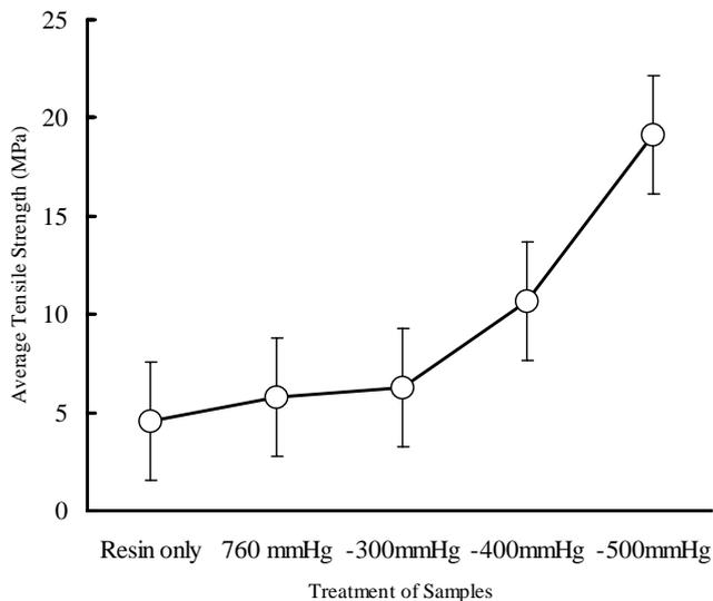
Figure 2. Average tensile strength of sago fiber composite.
