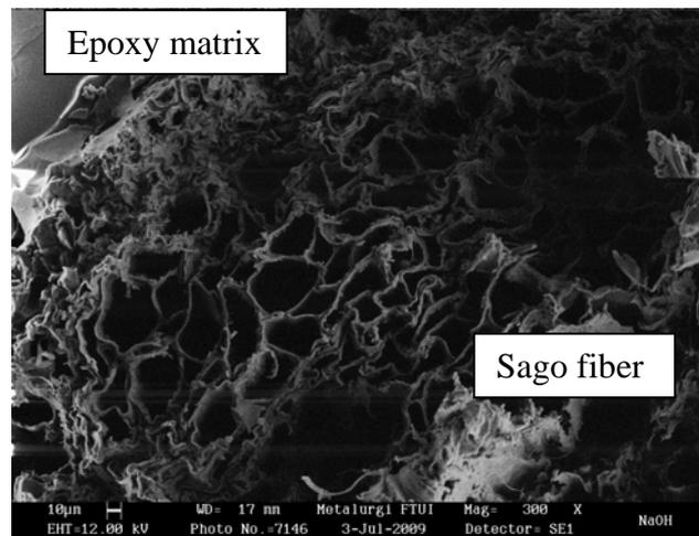
Figure 4. SEM fracture surface of sago fiber composite manufactured by vacuum.
