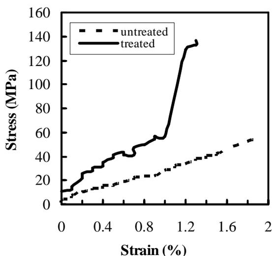
Figure 1. Stress-strain curve of a sago palm fiber in treated and untreated condition [2].
