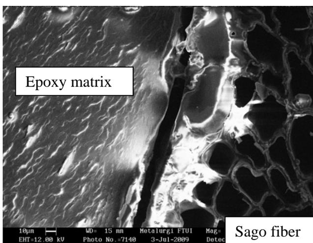
Figure 3. SEM fracture surface of sago fiber composite manufactured by non vacuum.
