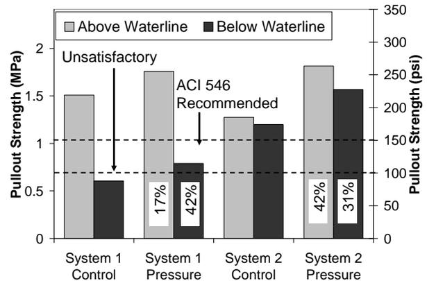
Fig. 2 Bond values from pullout tests for Scheme 2.
