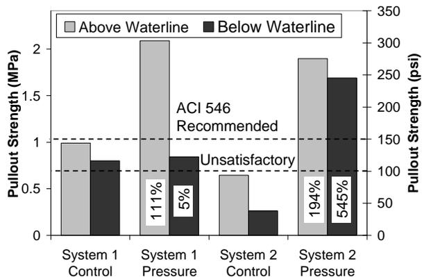
Fig. 1 Bond values from pullout tests for Scheme 1.
