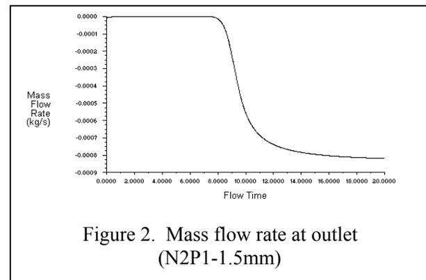
Figure 1 & 2 provide the resin mass flow rate plots with respect to flow time obtained by the 3D multiphase model RTM flow simulation for N2P1 sample with 1.5mm spacer thickness. It
