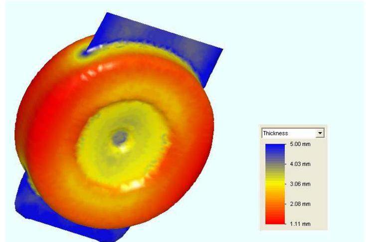
Figure 4: Thickness profile in the blow molded wheel (Perdikoulis, 2009; Garg, 2009)
