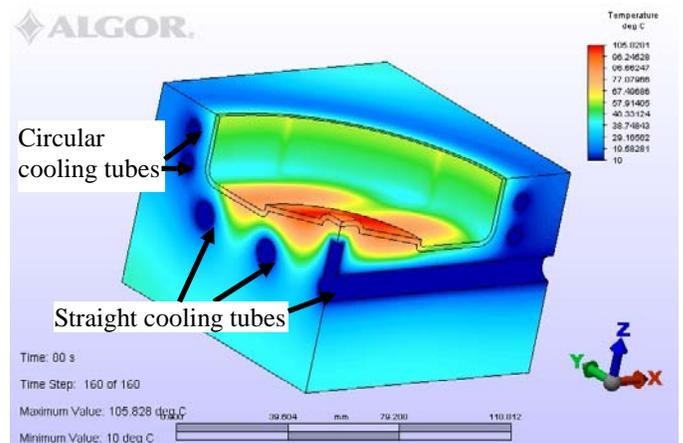
Figure 2: Thermal simulation of one quarter of the mold (Source: Garg, 2009)
