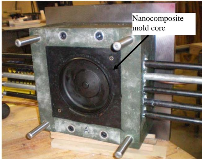
Figure 3: (b) Picture of one half of the fabricated mold with the nanocomposite mold core. (Source: Garg, 2009)
