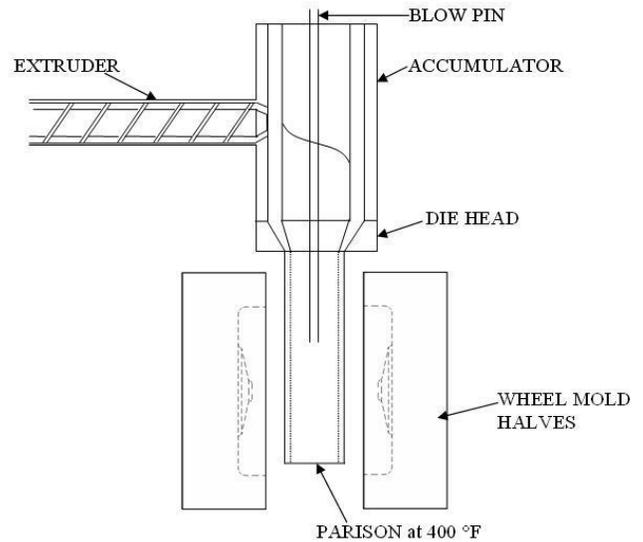
Fig 1: Schematic of Extrusion blow molding for a plastic wheel, showing the extruder, the parison and the two mold halves (Blow Molding, 2006; Alam et al., 2009)
