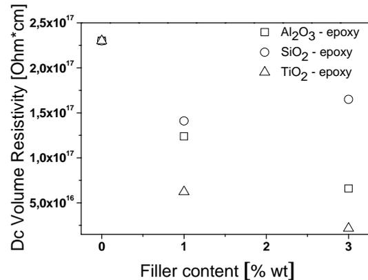
Figure 2. dc volume resistivity of epoxy nanocomposites.
