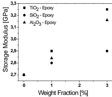
Figure 1. Storage Modulus of epoxy nanocomposites.
