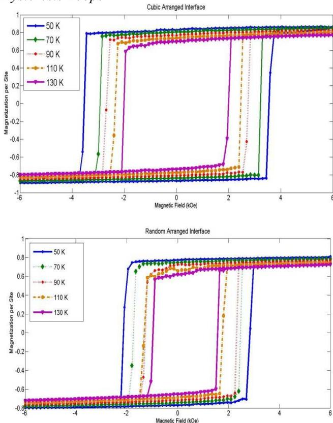
Fig 3. Hysteresis Loops at different cooling temperatures for CAI (up) and RAI (down)
