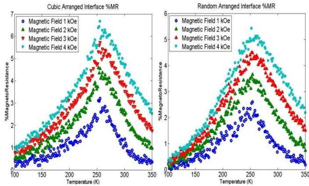
Fig. 2 Magnetoresistance vs Temperature: MR effect in Cubic Arranged Interface (CAI) (left) and Random Arranged Interface (RAI) (right)
