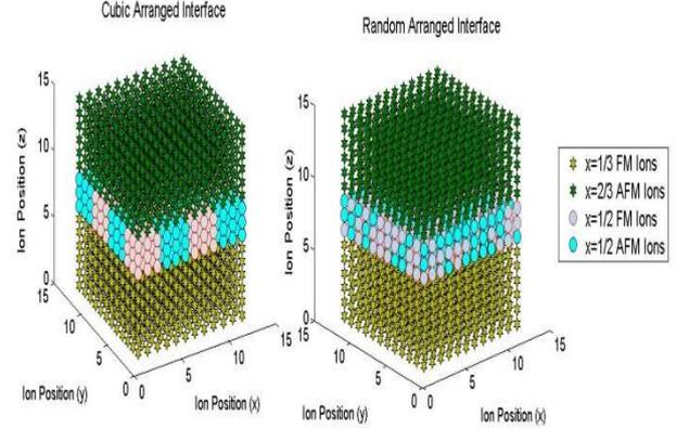
Fig. 1 Bilayer Construction: First layer of FM  $\text{La}_{2/3}\text{Ca}_{1/3}\text{MnO}_3$  phase, upper layer of AFM  $\text{La}_{1/3}\text{Ca}_{2/3}\text{MnO}_3$  phase. Cubic Arranged (left) and Random Arranged (right)  $\text{La}_{1/2}\text{Ca}_{1/2}\text{MnO}_3$  with FM and AFM phases put together.
