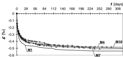
Fig. 2 Development over time of the autogenous shrinkage of the investigated composites.
