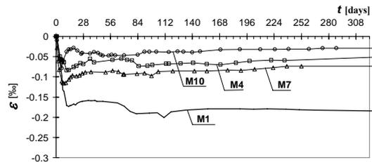
Fig. 4 Development over time of the drying shrinkage of the investigated composites.
