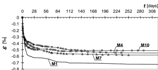
Fig. 3 Development over time of total shrinkage of investigated composites.
