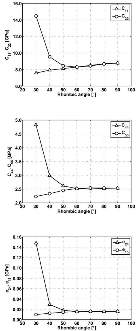
Fig. 2 Orthotropic behavior in transverse plane plotted for appropriate elastic and piezoelectric coefficients vs. change of rhombic angle with fixed fiber volume fraction of 0.4
