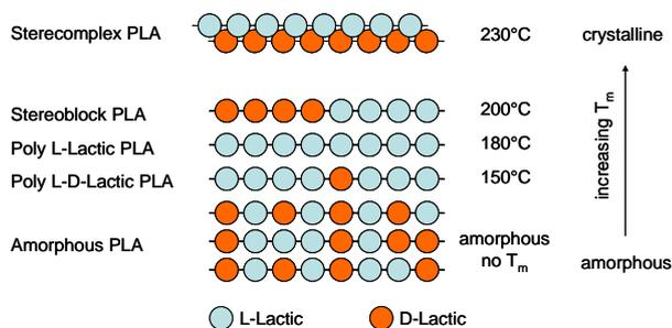
Figure 1: Dependence of the PLA melting point in relation to its chemical structure [2].
