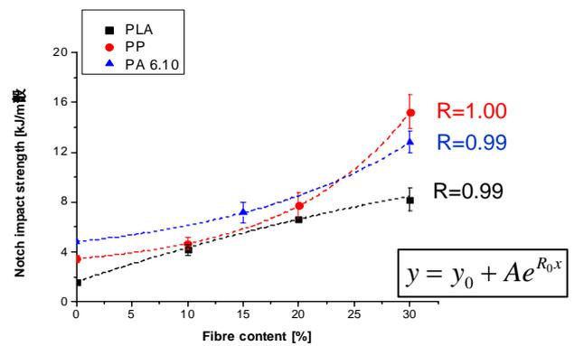
Figure 4: Charpy A-notch impact strength of man-made composites; testing temperature +23 °C.
