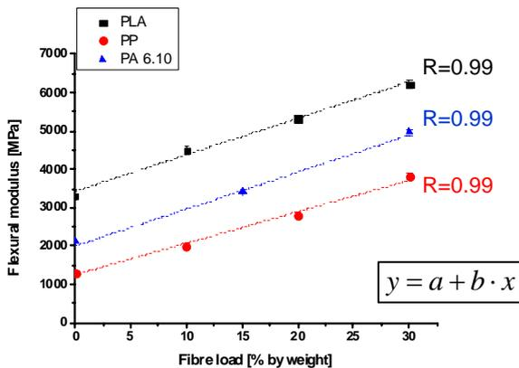
Figure 2: E-modulus of biocomposites with man-made cellulose fibres.
