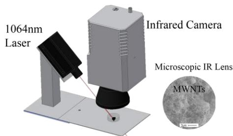
**Fig. 1.** Schematic of experimental setup. Only one laser is shown, but for the 650 nm tests the 4 lasers were symmetrically placed on all sides of the target area.
