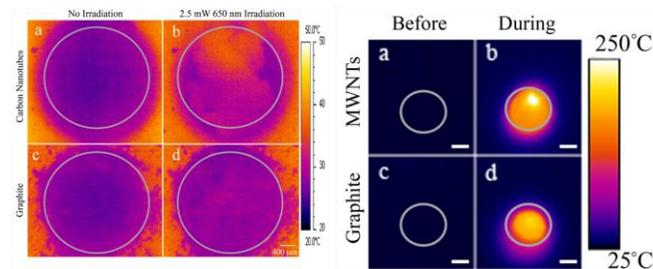
**Fig. 3.** Infrared images before (a,c) and during laser treatment (b,d) with four 650nm-2.5mW lasers (left) and a 1064nm - 320 mW laser (right). Images are of MWNTs (a,b) and graphite (c,d); target area inside circle (scale bars in the lower right corners of right image are 4 mm). MWNT temperatures exceeded the 265°C limit for the normal range of the infrared camera
