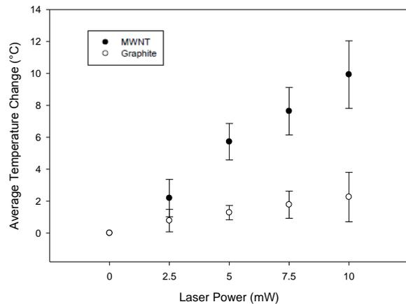
**Fig. 2.** Average maximum temperature increase above baseline of MWNTs and graphite vs. power while being treated with four 650 nm-2.5 mW laser sources in succession (mean  $\pm$  std).
