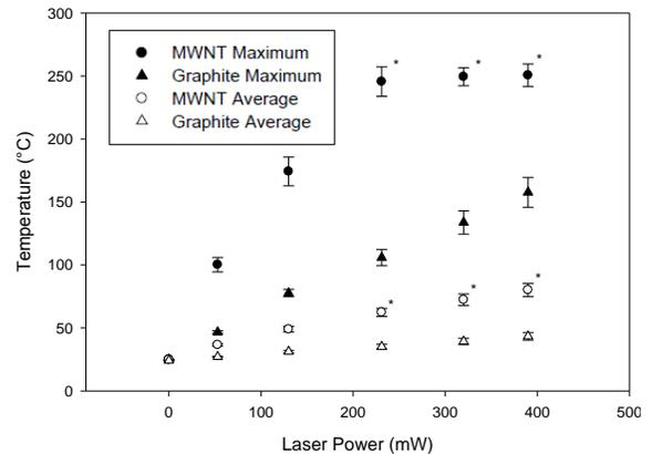
**Fig. 4.** Maximum and average temperatures as a function of laser power level. \*Actual temperatures above detection limit of 265°C
