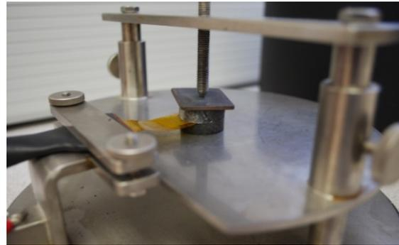
Fig. 4 Thermal Conductivity test setup.
